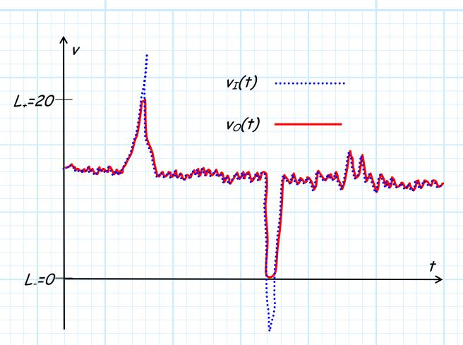
Note there are a couple of "hiccups" in the input voltage that take the voltage value outside the "safety" range of the sensitive device. However, the limiter does in fact limit these excursions, such that the voltage across the sensitive device always remains between 0 and 20 Volts.
